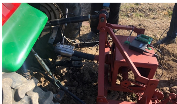
Figure 1. TRA-50K resistance strain gage installed between the tractor PTO shaft and bevel gear speed inducer shaft of the tiller.
