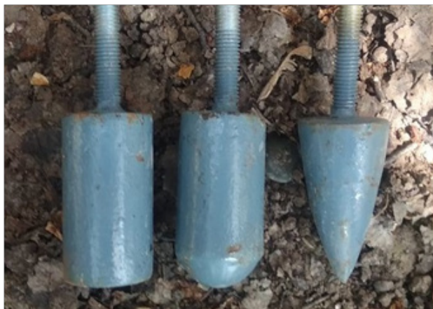
Figure 2. The experimental fingers of the clod-crusher in the potato digger.
