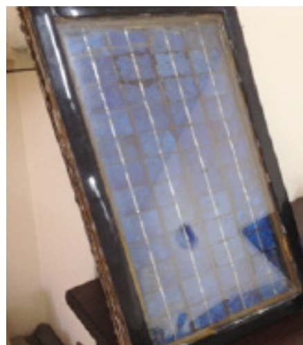
Figure 3. Desalination device with integrated PV panel.
