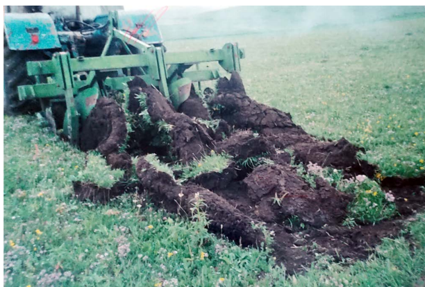
Picture 1. Field testing of the frontal plough on a slope without reversible plowshares.
