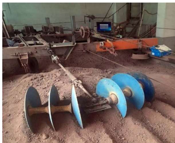
Picture 2. View of the disc battery of the combined machine captured from laboratory and field experiments.
