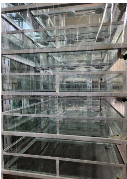
Picture. Cuboid cell photobioreactor (photo and general layout of structured designed and constructed in the company). 1- The metallic frame of a photobioreactor, 2- plain glass, 3- LED lighting system (composed by the authors).
